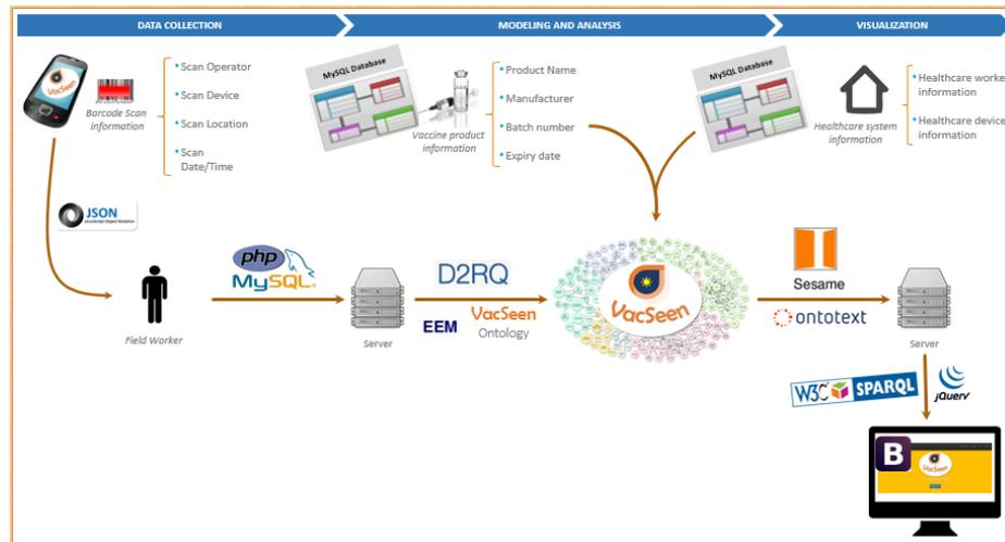
Fig. 1: The VacSeen project - System Architecture
